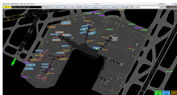
Figure 3. Ramp Manager Traffic Console (RMTTC).
