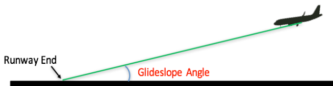
Figure 6. Diagram of glideslope angle
