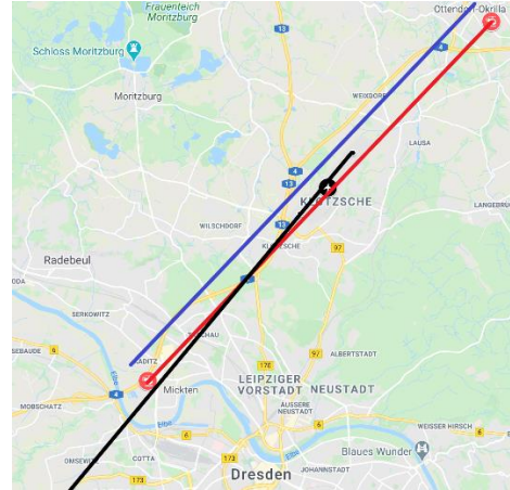
Figure 10. Use case Scenario, drone leg (red, baseline/blue, offset scenarios), linking two drone parcel stations, crossing DRS final approach track (black)
