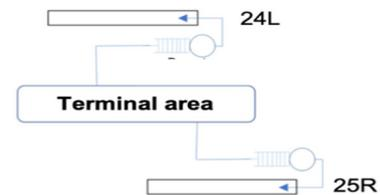
**Figure 6. LAX Taxi-out Queuing Network Representation (West-Flow Configuration)**
