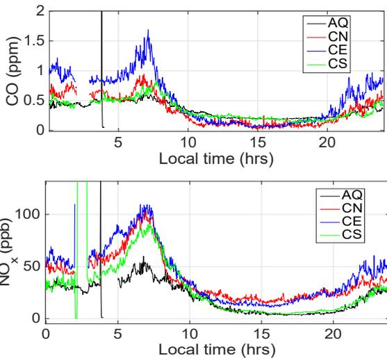
**Figure 12. Pollutant Concentrations of CO and NO<sub>x</sub> at the Four Emissions Monitoring Sites**
