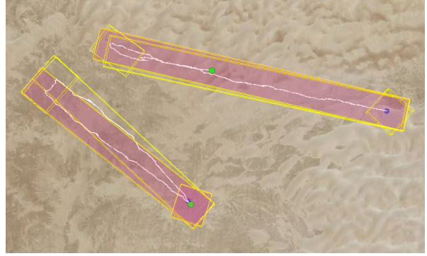
Figure 3: Example out-and-back operations with the white completed flight track and green vehicle position shown within the yellow planned operation volumes, and red active volumes.
