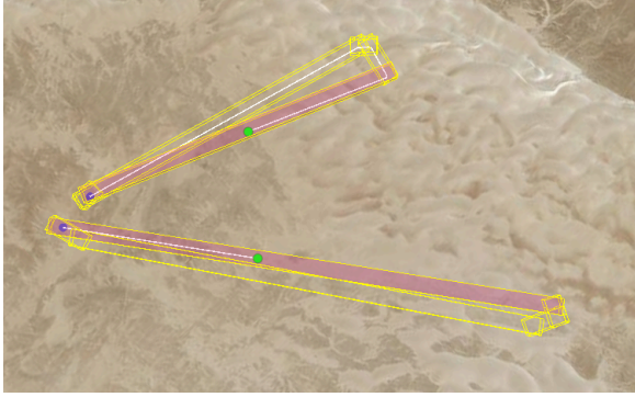
Figure 3: Example out-and-back operations with the white completed flight track and green vehicle position shown within the yellow planned operation volumes, and red active volumes.
