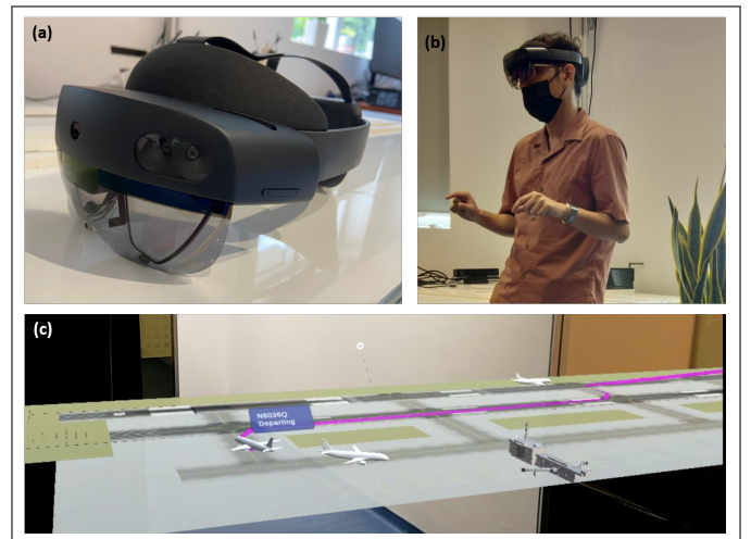
Figure 1: (a) Microsoft HoloLens 2 (b) An Air Traffic Controller wearing the HoloLens 2 (c) The DT simulation in Mixed Reality with overlaid aircraft billboards.
