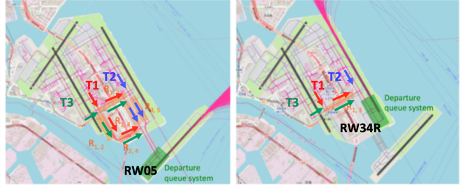
Figure 5: BSRs at RJTT. BSRs are shown in rectangles connecting BIAs with departure traffic flows from each the terminal.
