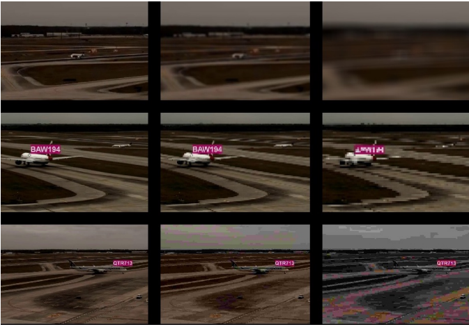
Figure 2: Synthesized low-fidelity samples. Left to right: clean, corrupt level 1 and corrupt level 3 samples. Top to bottom: blurring, pixelating and JPEG compression.
