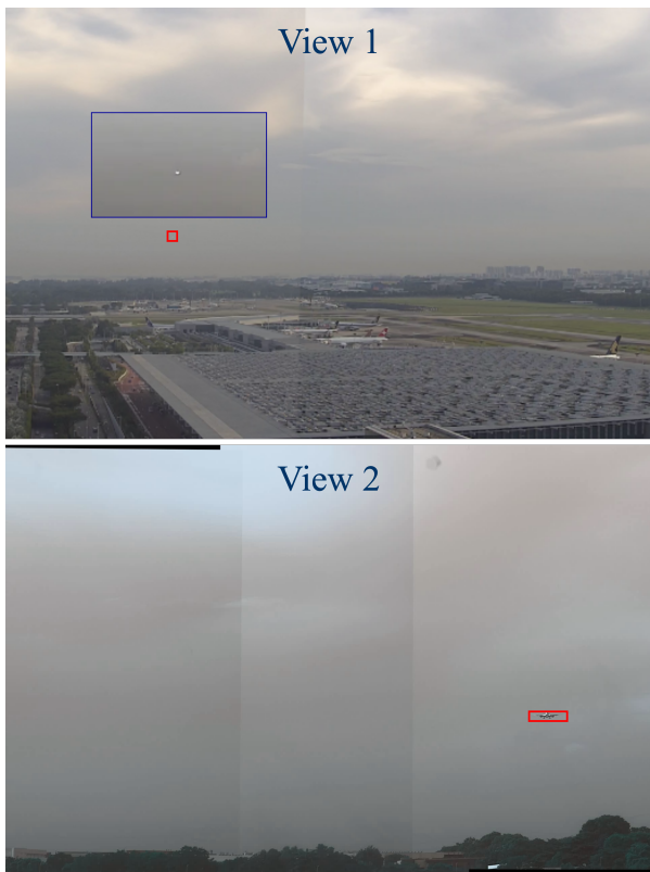
Figure 10: An example of video data from Changi Airport. View 1 is from the camera mounted on the top of the control tower, while View 2 is from the camera at the LLZ hut. The red rectangles highlight the position of the aircraft in their respective frames. The image segment with a blue border in View 1 is the zoom-in for better observing the small aircraft.
