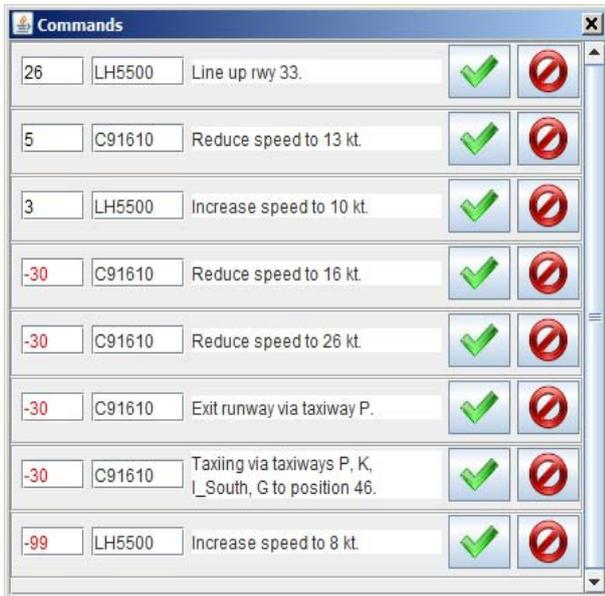
Figure 2. Controller Command Panel. For each aircraft the time in seconds until activation, aircraft-ID, command and accept and reject buttons are shown.
