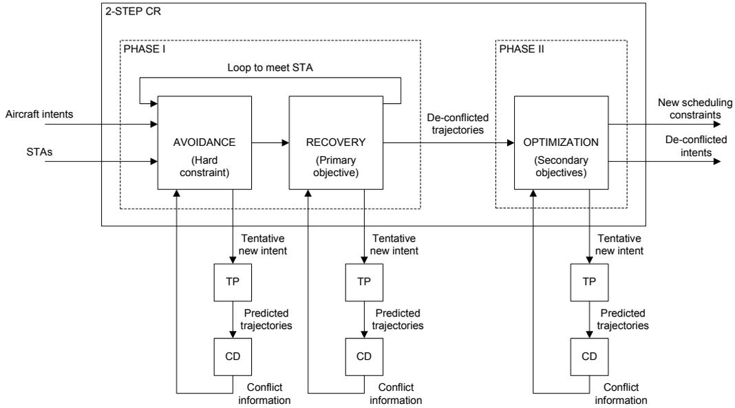
Fig. 1. Structure of the 2-step CR algorithm.
