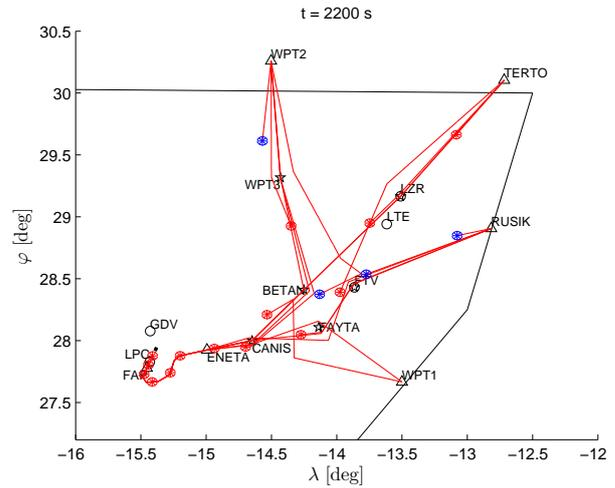
Fig. 8. Scenario 2, 3-step CR resolution trajectories at  $t=2200$  s.
