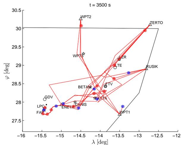
Fig. 9. Scenario 2, 3-step CR resolution trajectories at  $t=3500$  s.
