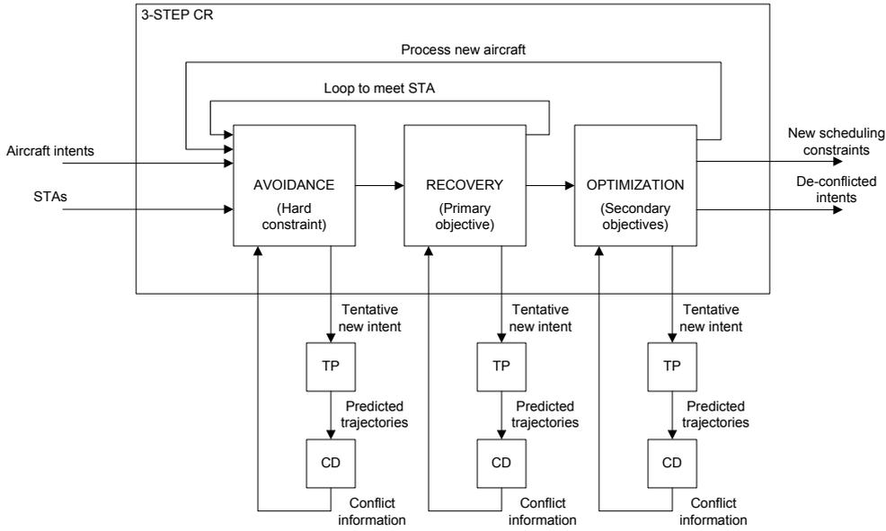
Fig. 2. Structure of the 3-step CR algorithm.
