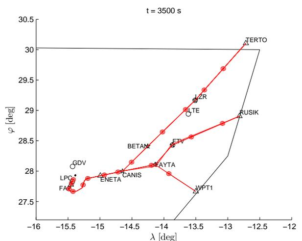
Fig. 6. Scenario 1, 2-step CR resolution trajectories at  $t = 3500$  s, Phase 2.
