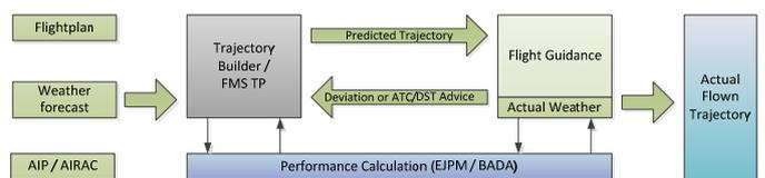
Figure 4: TABATS Schematic Simulation Process
