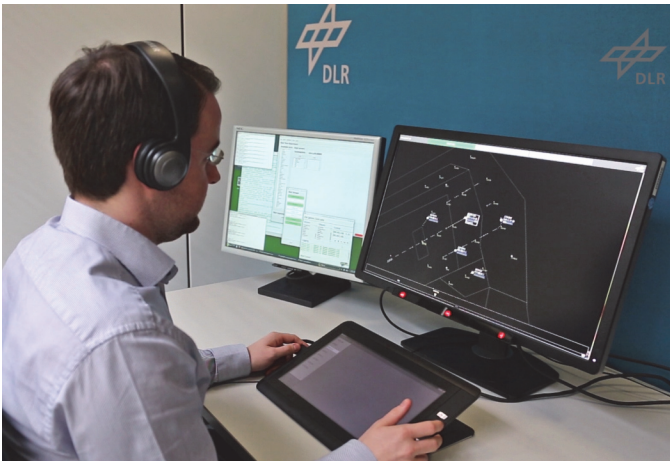
Figure 7. TriControl setup with radar display attached eye tracker, headset, and multi-touch device
