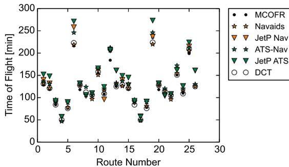
Figure 4. Time of flight of 13 simulated trajectories on daytime (Routes No 1 to 13) and night time (Routes No 14 to 26) following different target functions. In general, conventionally filed trajectories (JetPlan.com) result in long flight times, whereas multi-criteria optimized trajectories are the fastest.
