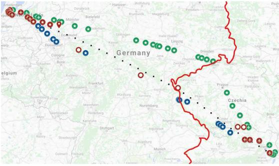
Figure 6. Different ConOps simulated for the city pair Amsterdam (EHAM) to Vienna (LOWW), route No 9 at night with FRA implementation (DCT in FABEC) in ConOps 4 (ATS ORANI, red) and ConOps 6 (TOMATO ATS route, blue). Black dots: MCOFR (ConOps 1), green stars: Airways optimized route from JetPlan.com (ConOps 5) red circles denote E and EXI wp. The red line indicates the FABEC boundary.
