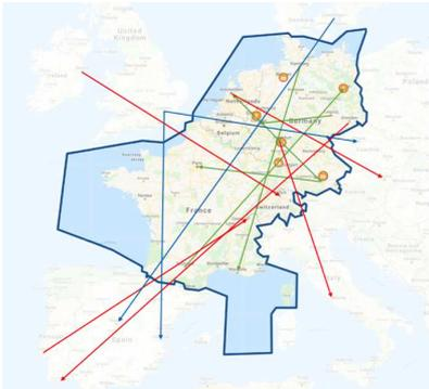
Figure 1. Overview of simulated city pairs in this case study in FABEC (blue polygon). Colors indicate trajectories within FABEC (green), with either departure or destination outside FABEC (red) and with both airports outside FABEC (blue).
