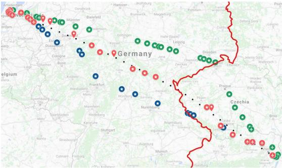
Figure 7. Trajectory optimization between Amsterdam (EHAM) and Vienna (LOWW), route No 9 at daytime without DCTs in FABEC. Green: JetPlan.com, airways optimized. Blue: TOMATO ATS-Route. Red: ORANI ATS with Nav aids, from which red stars are waypoints along an ATS route, red markers indicate waypoints of the navaid infrastructure and red circles denotes E and EXI wp. The red line indicates the FABEC boundary.
