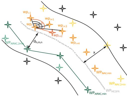
Figure 2. Procedure of ORANI's waypoint adaption of MCOFR (grey) to the navaid infrastructure (yellow) and to the ATS route structure (turquoise), after filtering the solution space (Eq. 7) and large heading changes ( $\beta$ ).
