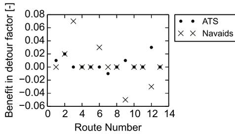
Figure 3. Benefit in detour factor due to implementation of DCTs in FABEC for flights at nights. Positive values denote shorter ground distances with FRA implementation in FABEC. Dots correspond to ConOps 4, crosses denote ConOps 2. The corresponding city pairs are listed in Table II.
