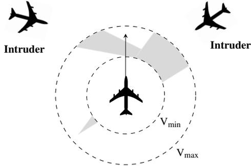
Figure 4. SSD resolution. Adapted from Dam [13].
