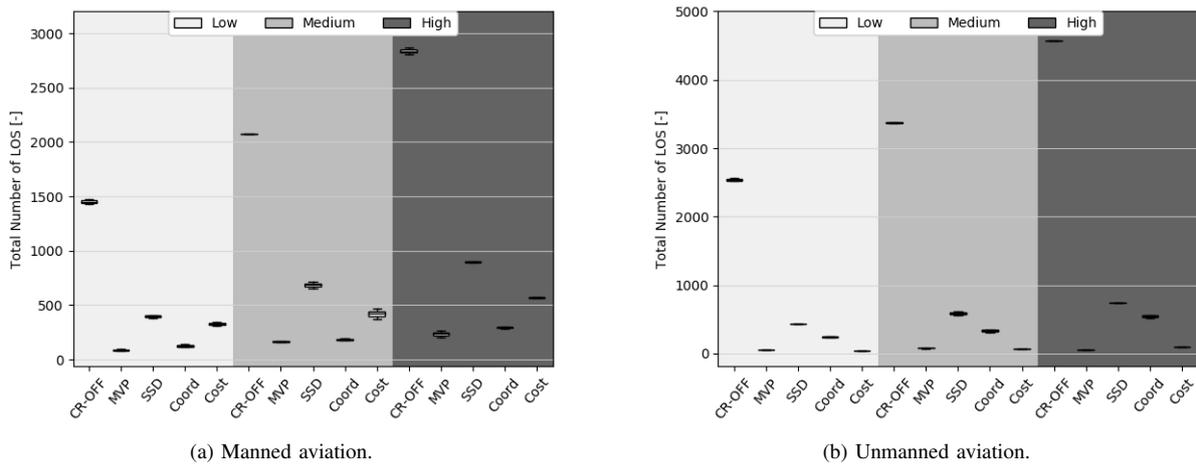
Figure 8. Number of losses of separation per CD&R model.
