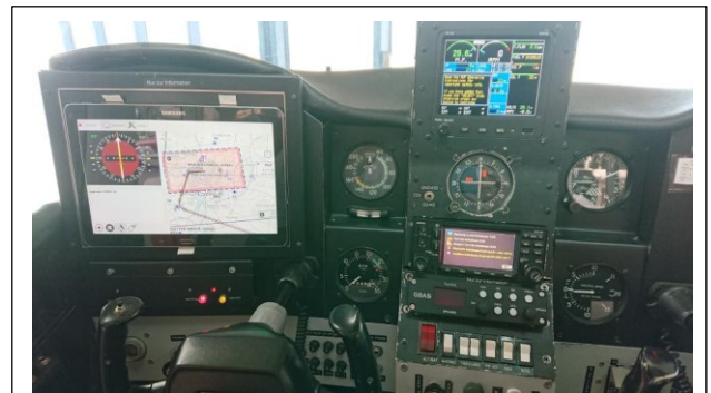
Figure 2. Cessna 172N cockpit installations with navigation prototype on portable display TUBS (left) and COTS instrumentation
