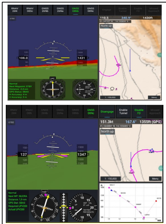
Figure 5. CIRA/NAIS pilot's HMI for first RTS campaign (top) and the second RTS campaign (bottom).
