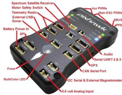
Figure 6. AIRCATEC Pixhawk autopilot.
