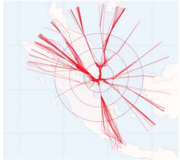
Figure 11. One day examples of flight track data arriving at Singapore Changi International Airport within 500 NM radii concentric circle centered at the airport.
