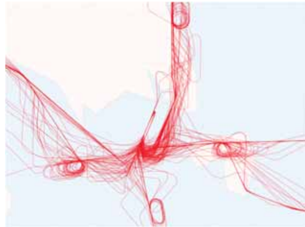
Figure 12. One day examples of arrival tracks around Singapore Changi International Airport, emphasizing holding areas.
