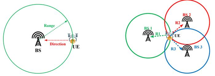
Figure 4. (a) Single Base Station Positioning Scenario; (b) Multi-Base Station Positioning Scenario
