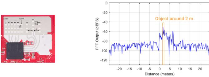
Figure 15. (a) AWR1843 board, TX and RX antennae details [25]; (b) 1D FFT amplitude profile (per chirp)
