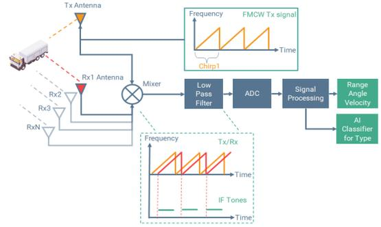
Figure 6. mmWave radar architecture with multiple Rx Antennae
