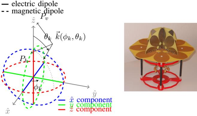
Figure 2. (a) Topology of a theoretical VA; (b) Photograph of the 8-port vector antenna [14]
