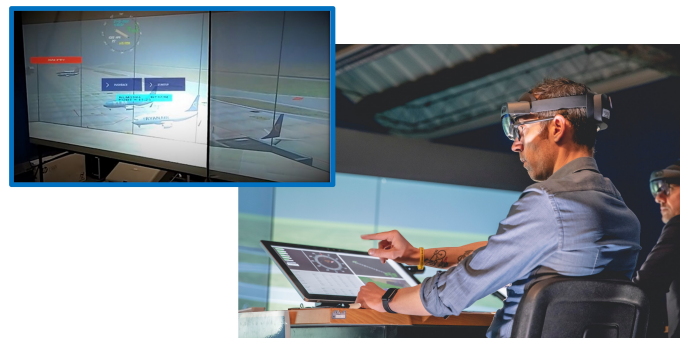
Figure 8. VAR-002 Air Gestures solution exercise: ATCOs can simultaneously see both the out of the tower view and the AR overlays through HoloLens2. The personal view of the GND controller who is interacting with the overlays is depicted in the blue square.
