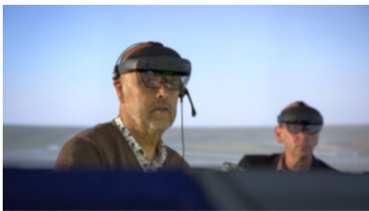
Figure 9. Tower Controllers with HoloLens2 (NARSIM).
