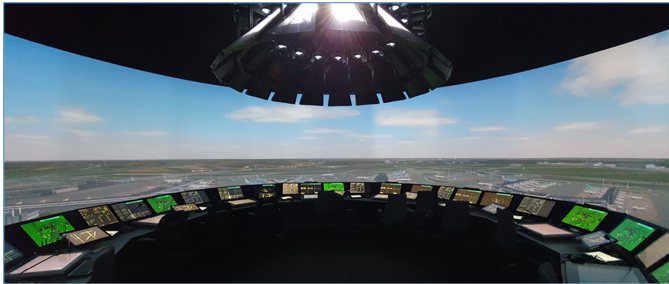
Figure 1. NARSIM Tower Validation Platform at NLR Amsterdam.
