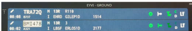
Figure 1. Callsign highlighting (white box around "BMI478") and automatically recognized flight status change from voice utterance (dark green "TAXI" via "C") on the electronic flight strip display's ground bay as well as earlier clearances (light green STARTUP, PUSHBACK).
