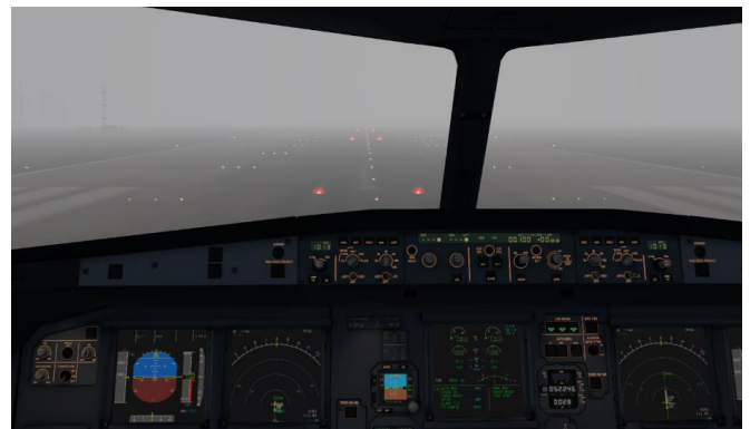
Figure 2: View from the cockpit to the Take-off Support Lights at poor visibility (aircraft model by ToLiss Simulation Solutions Inc.)
