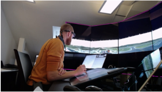
Figure 1. The MRTO simulator environment consisting of one large display, with optical sensor presentation (OSP) split to show the 360° camera feed from both airports, one radar display for each airport to the left and right of the ATCO, respectively, and a split digital flight strip display in between. Here the right radar display has been replaced by our DiTA display. Also, only one OSP presentation, indicated by a purple border, is visible in the photo due to its angle.
