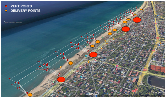
Figure 2. Corridor-based airspace structure used in the Spanish demonstrations in the CORUS-XUAM project
