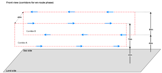
Figure 3. Concept view of the four corridors to be used in the simulation scenario.
