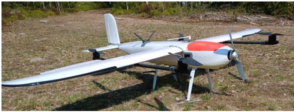
Figure 1. Loong 2160 drone with the antennas placed on the front top, rear bottom and legs of the landing gear.
