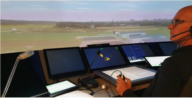
Figure 4. NARSIM Tower Control Room for EHRD with CAUSIC Display
