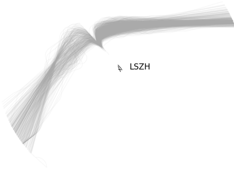
Figure 3: Trajectories landing at Zurich airport, runway 14
