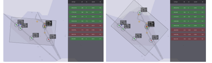
Figure 7. Changing the orientation of the rectangle (major axis) is done by adding only one flight (QFA24B, upper right), which in this case also halves the complexity value.
