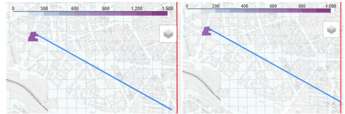
Figure 11. Results for VP-4 indicators for inbound and outbound trajectory at the same altitude (visible area metric). Left: inbound flight. Right: outbound flight. Altitude 66 m.
