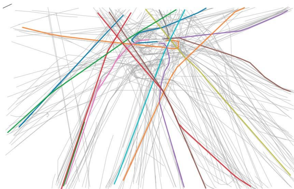
Figure 2: Clustering of ADS-B data to define ATM flows – Source: OpenSky and DBSCAN
