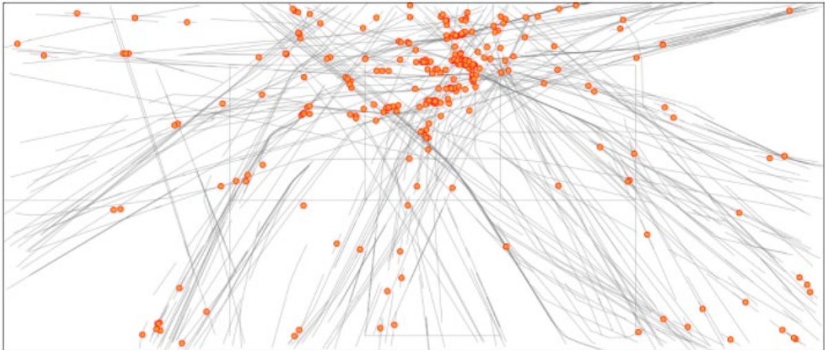
Figure 3: Highlight of "hotspots" over ADS-B flows intersection points – Source: OpenSky and DBSCAN
