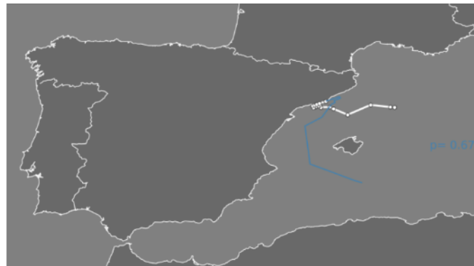
Figure 19: FP (white) and DIAPasON prediction (blue) 4 hours before EOBT for flight #3229838 LIRF – LEBL.
