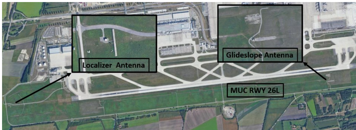
Figure 41: The locations of the ILS antennas of Runway 26L in Airport 2 on Google Maps. [30]
